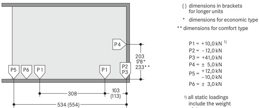
Bearing loads are transmitted by wall plates with min. 30 cm<sup>2</sup> surface and to the floor by base plates with min. 350 cm<sup>2</sup> surface.
